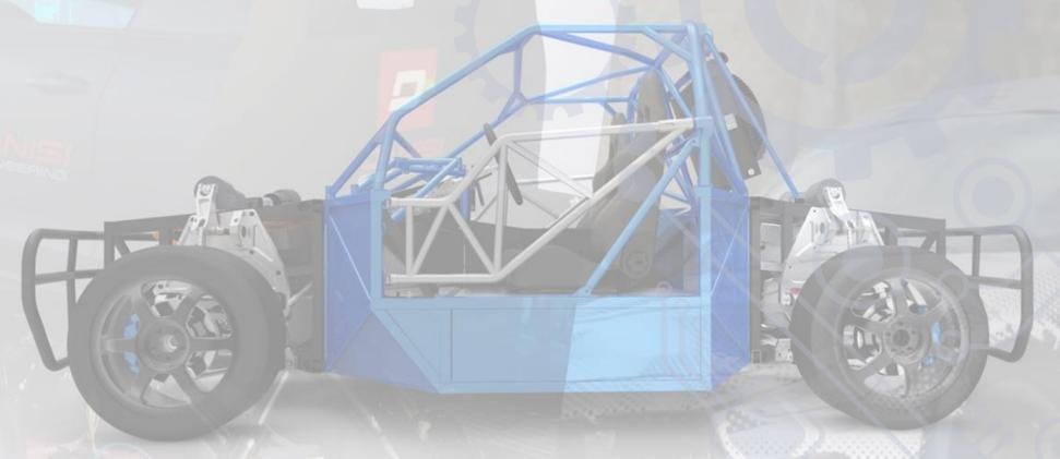
MRP can be used for developing new cross-domain functions for all present and future vehicle concepts. As a completely open platform, it makes possible the integration of almost any user-specific hardware and software components.
